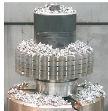
Clamp nut clamping sprockets during milling
